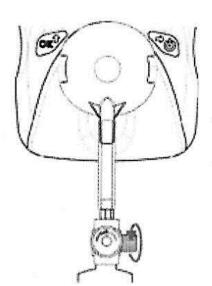
2. Enter the calibration function, open the gas cylinder, press the Left Key, and start calibration after countdown.
