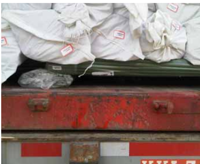
Figure 5-5-2 Example of Inadequate Spacing Under Bamboo Bundles
